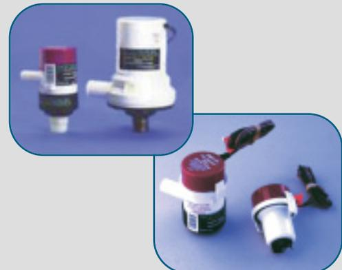
Kodiak's new cartridge-style pump shown to the right is available in 2 sizes, K500C and K700C Thru-Hull Mount and KB500C and KB700C Transom Mount. The motor snaps out of the water jacket, allowing fast cleanout of weeds and easy "on the water" replacement.
